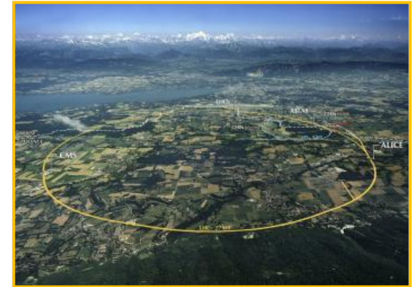
Large Hadron Collider 27 km, 8.33 T, 14 TeV 1300 tons NbTi
