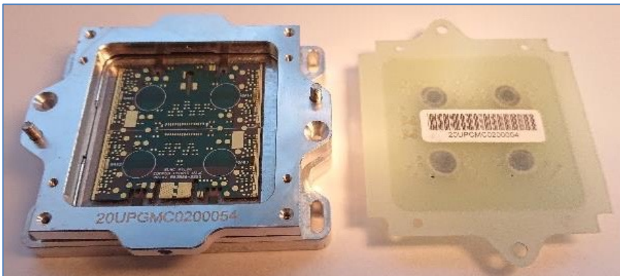
Prototype module for layer 1-4 quad module in carrier for testing and transport
