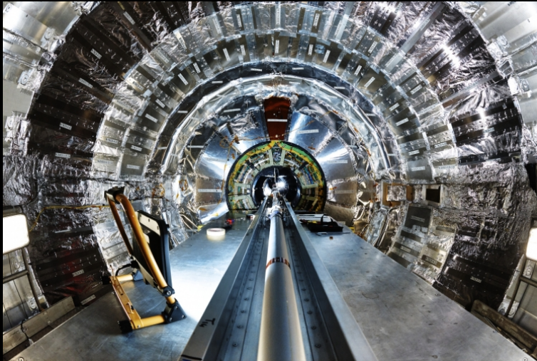
Installation of new beampipe
