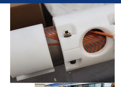
prototype Q1 canted cosine theta with fringe field correction, using LHC SC cable
