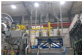
Silicon beam telescope mounted next to the target loading platform to test the refurbished \text{LN}_2 cooling.
