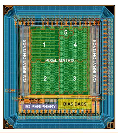
ASIC prototype with 12x12, 65µm side hexagonal pixels with 80fF capacitance come in different "flavors":
