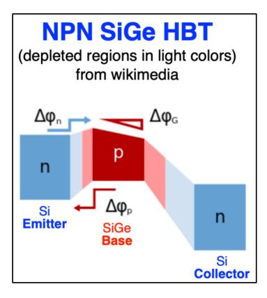
SiGe Hetero Bipolar Transistor (HBT) = Bipolar Junction Transistor (BJT) with Germanium in base material:
