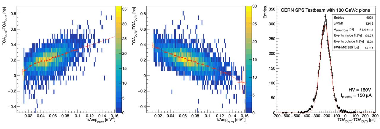
• Correction performed with respect to inverse of signal amplitude for both DUTs.
