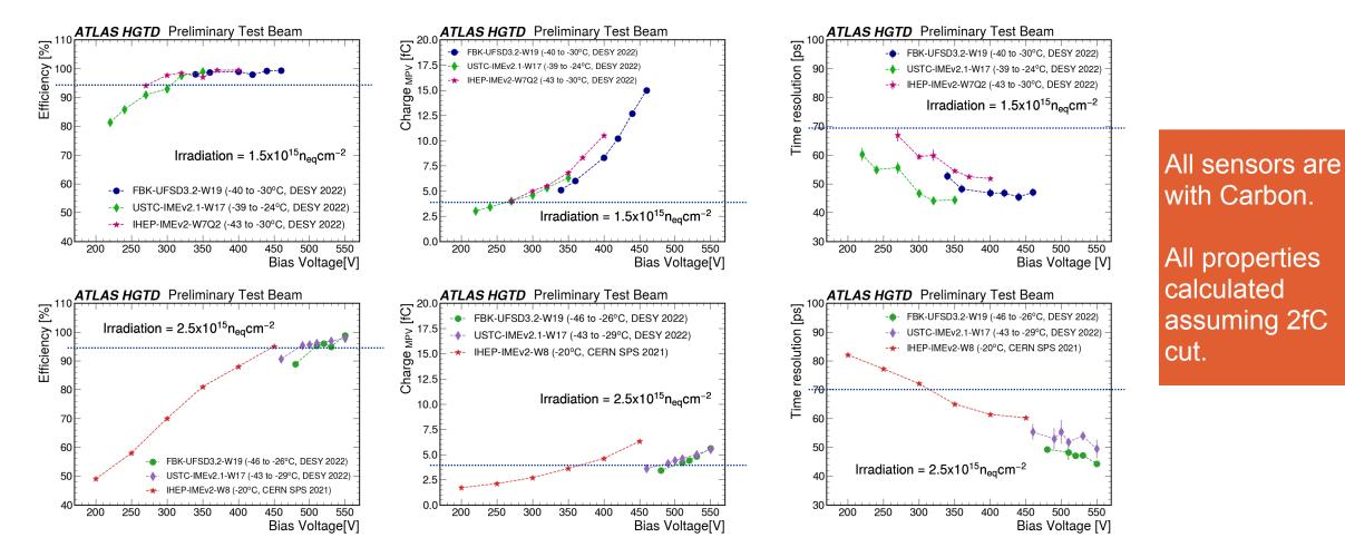
At highest biases, DUTs irradiated up to 2.5E15, have efficiency > 95%, charge > 4 fC and time resolution < 70 ps. **Meet HGTD specifications !**
