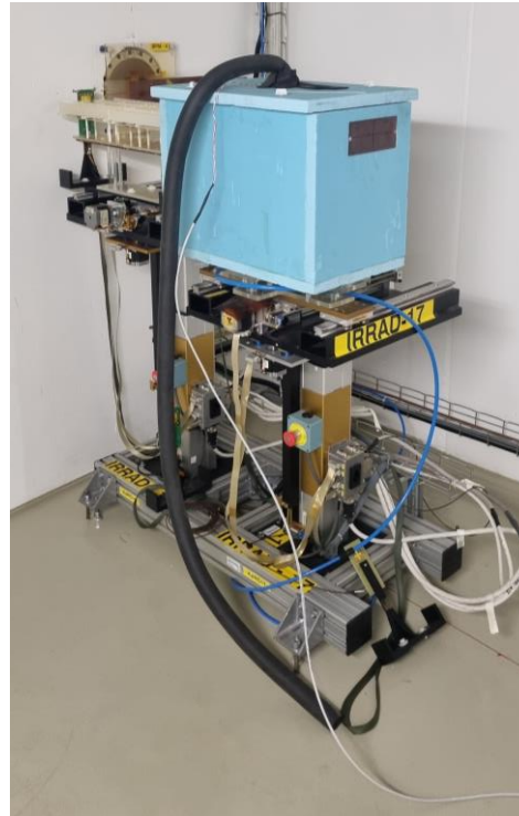
IRRAD cold-box with VORTEX system for long-run experiments
