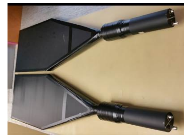
Beam Trigger (2 pairs of scintillators)
