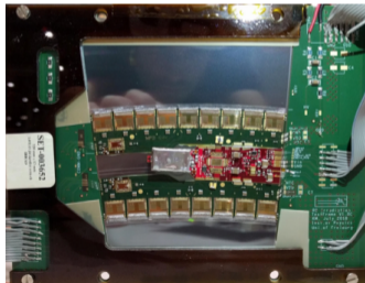
R0 module; neutron irradiated sensor, X-ray irradiated ASICs and powerboard.
