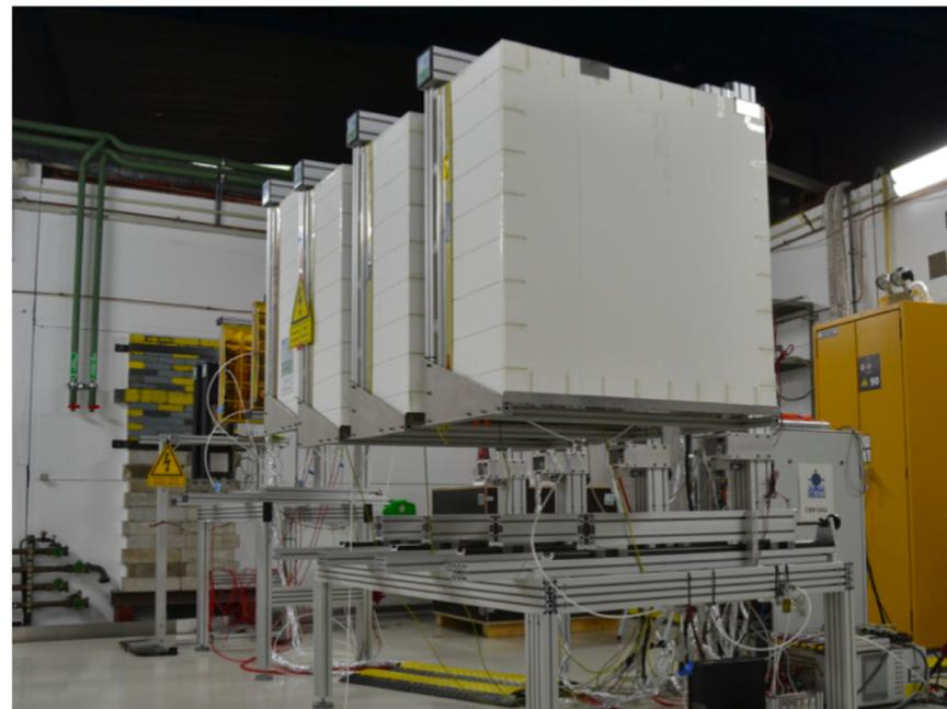
Test beam prototype of large chambers.
