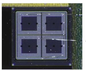
Irradiated 2x2 prototype array from FBK.
