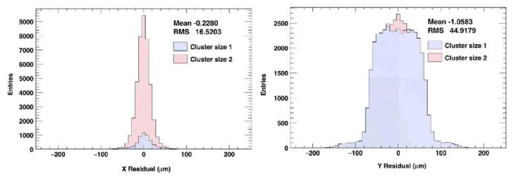
The projected resolution on the DUT is about 8um, measured on a 3D pixel detector.
