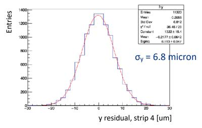
The mean projected resolution on the DUT is about 4um
