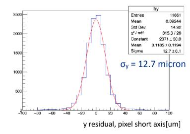
The mean projected resolution on the DUT is about 4um
