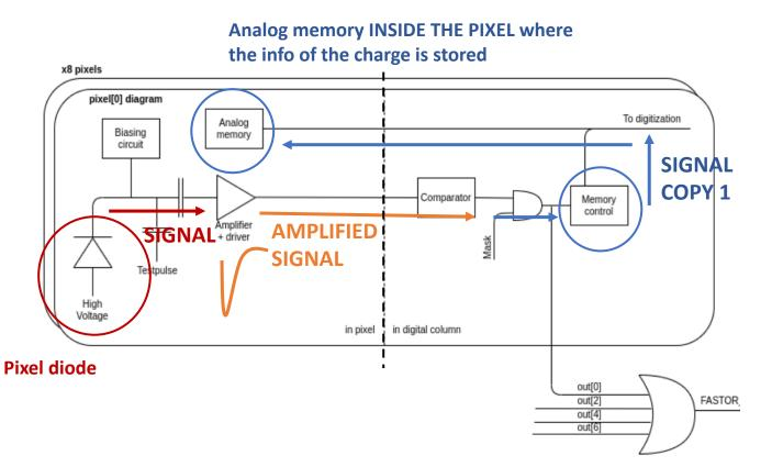
Memory Control loads the analog memory inside the pixel if the charge is over threshold
