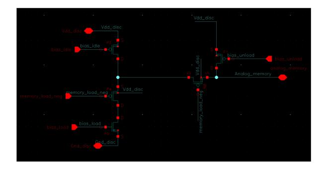
Current leakage even if the switch is opened. It takes 200 μs to degradate the memory value of 30 mV (= 1 bin of our ADC).
