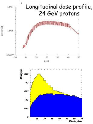
For comparison: longitudinal dose profile, LHCb, innermost cell (from TDR)
