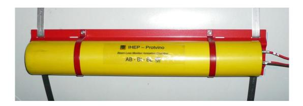
•Ionization chamber. No bunch by bunch possible respond time •LHC: Small IC (filled SEM) ~ 30 less sensitive than IC.
