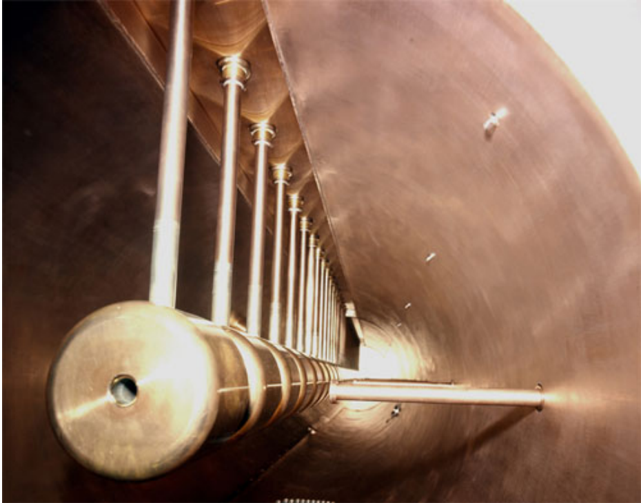
A detail of the LINAC2 drift tube (from here )
