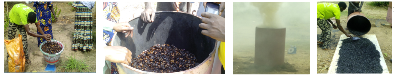
1. Weighing the raw material 2. The filling 3. Advanced charring 4. Material's withdrawal
