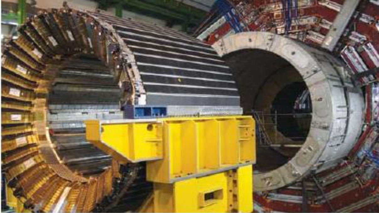
The CMS HCAL being inserted into the solenoid
