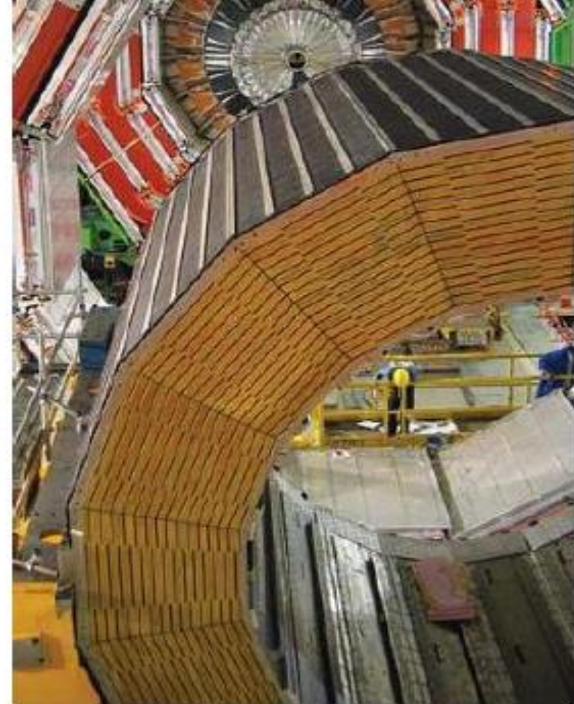
Light produced in the scintillators is transported through optical fibres to Hybrid Photo Diode (HPD) detectors
