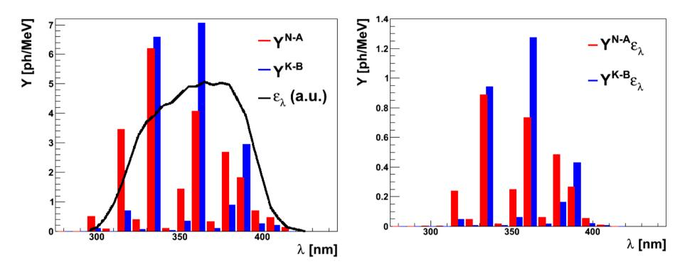
Fluorescence photons are detected with optical systems that have  $\lambda$ -dependent response (black line). When this efficiency is taken into account the relative intensities of the molecular bands are modified (right picture).
