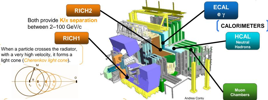
The **photosensitive surface** is designed to capture the particles' emission crossing the radiator. By measuring the angle,  $\theta$ , of the Cherenkov cone, RICH detectors extract the particle velocity.
