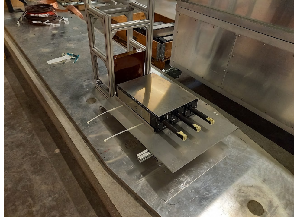
Calorimeter and preshower support
