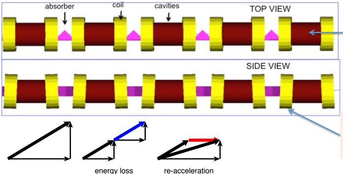
Limit muon decay, cavities with high gradient in a magnetic field tests much better than design values but need to develop
