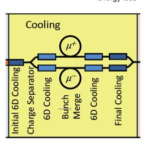
A few final cooling solenoids pushing to the absolute limit (30 - 50 T) Luminosity is proportional to field
