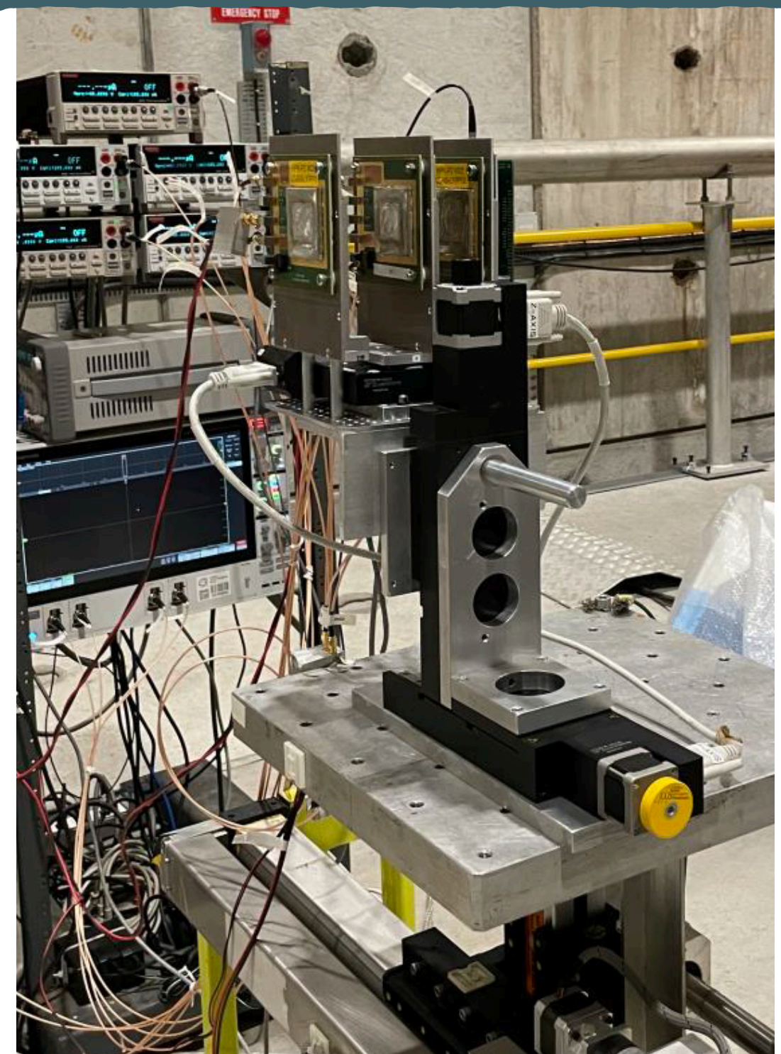
Test of timing sensors for VELO vs incidence angle
