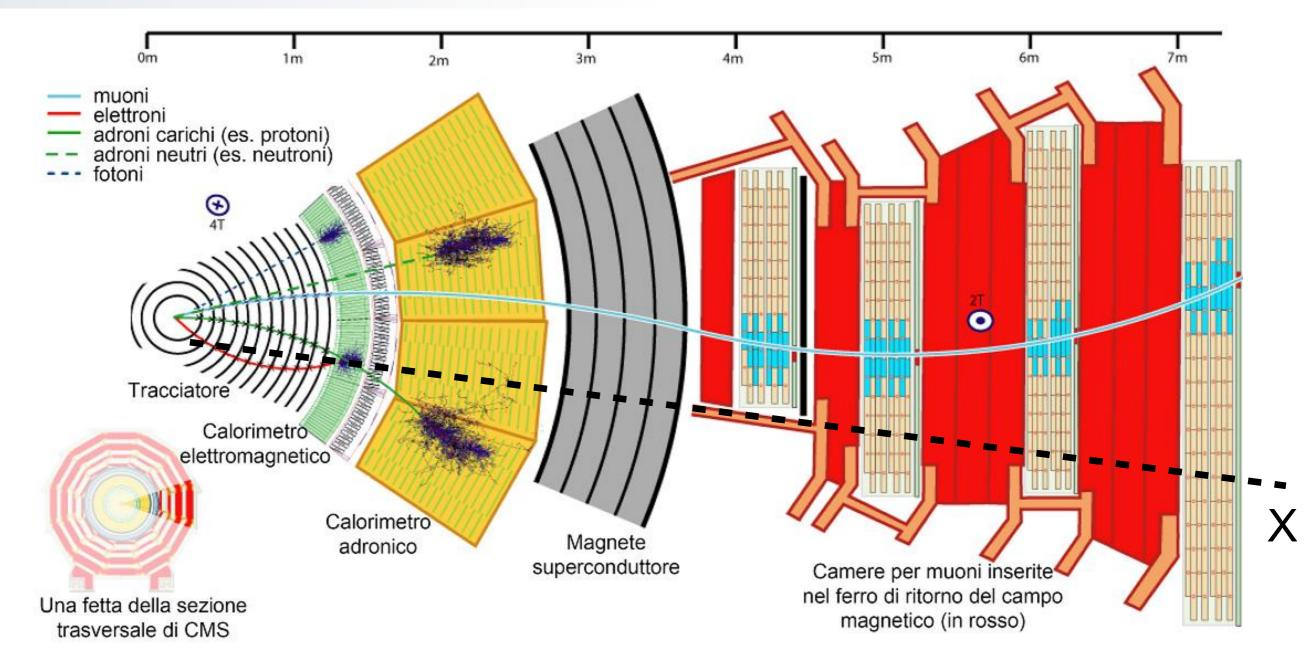
Detectors record signals from hadrons, charged leptons, and photons
