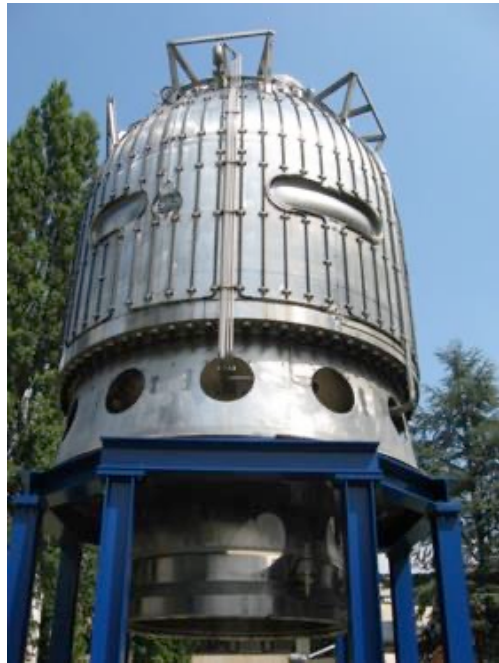
Big European Bubble Chamber 3T; L=3.5m, X_0=34\text{cm}
