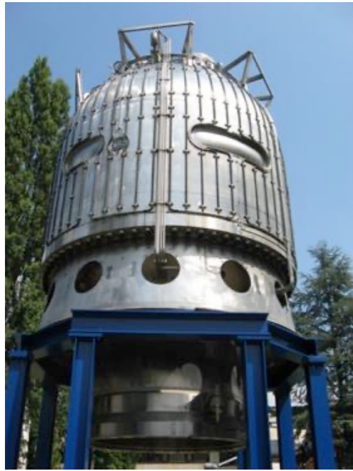
Big European Bubble Chamber 3T; L=3.5m, X_0=34\text{cm}
