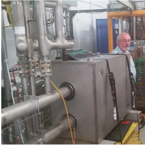
Test of fast-ramping normal-conducting magnet design
