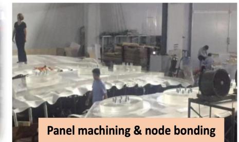
Panel machining & node bonding
