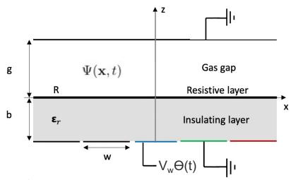
Weighting potential for only perfect insulators and electrodes with infinite conductivity.
