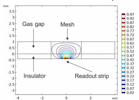
Weighting potential for a resistive layer separating the gas gap and insulating layer.
