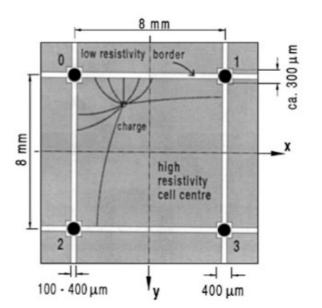
Time-dependent weighting potential map for one readout node
