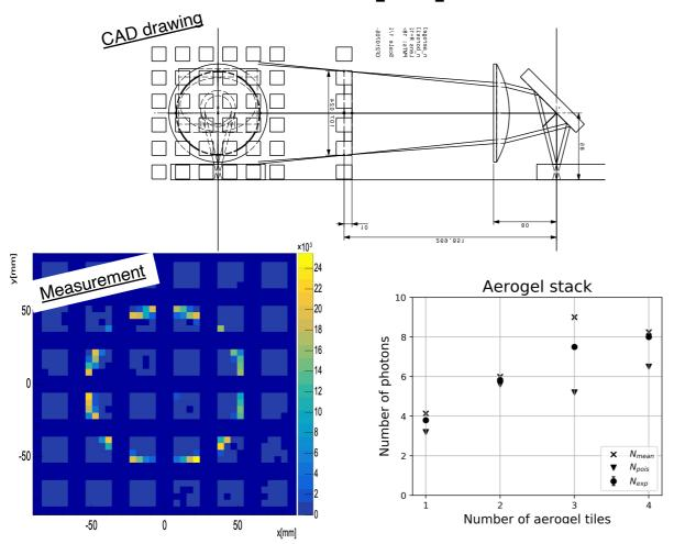
**Tentative/preliminary** results show high transparency (nearly linear for thicknesses up to 8 cm) and, taking into account various corrections, a yield of  $\mathcal{O}(65)$  photons / cm of aerogel.
