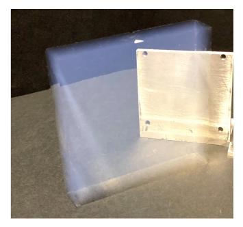
**Novel silica aerogel tiles** produced in Japan (<a href="https://arxiv.org/abs/1112.3121">https://arxiv.org/abs/1112.3121</a>). Hydrophobic and with improved transparency.
