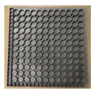
First flat carbon-fibre mirror prototype produced for RICH 1.
