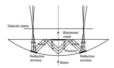
Coated lens was used to generate, reflect and focus the Cherenkov photons.
