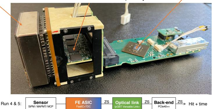
A new version of the chip, 'FastIC+TDC', is under development including internal digitisation with a TDC.
