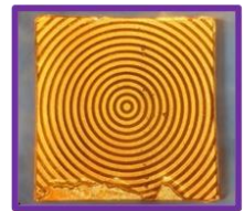
240 \mu m stripes 250 \mu m trenches 49% HTS
