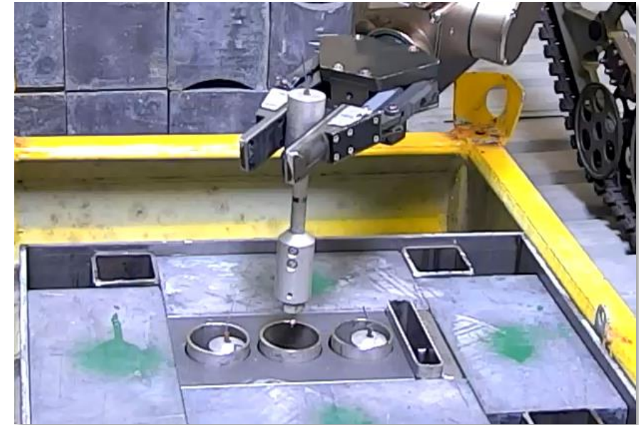
Radioactive sample handled by a robot
