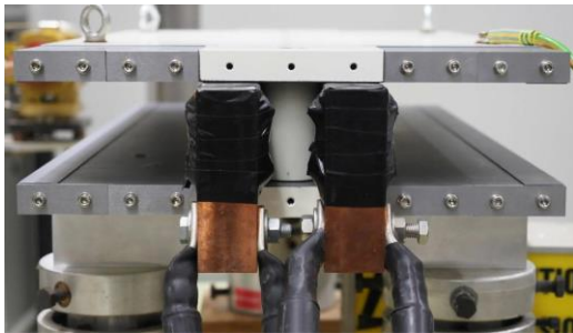
Prototype 1m-long, single busbar “coil”, measurements reported in [3]
