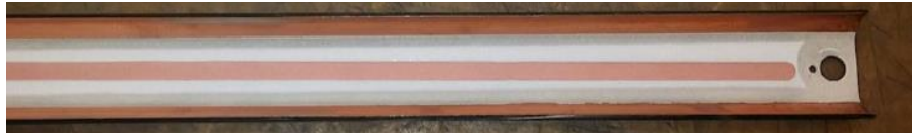
Copper and aluminium cold spray coating on ceramic insulated copper coated stainless steel sheet
