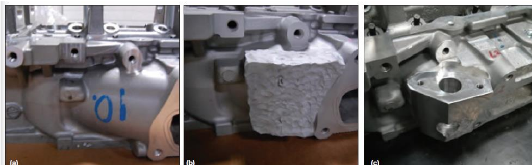
Fig. 3 — Freeform feature added to a prototype machine component by cold spraying. (a) Prior to spraying, (b) as sprayed, (c) finished.
