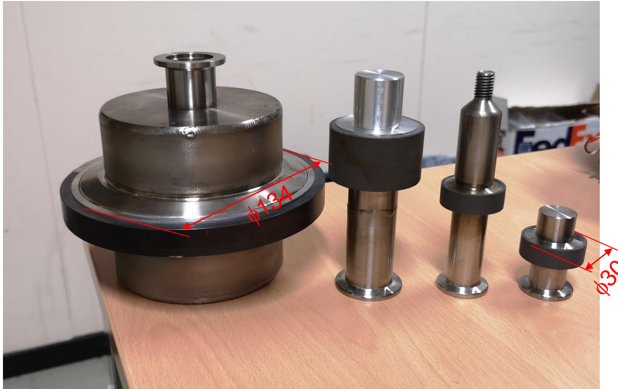
Examples of different validated SMA connectors
