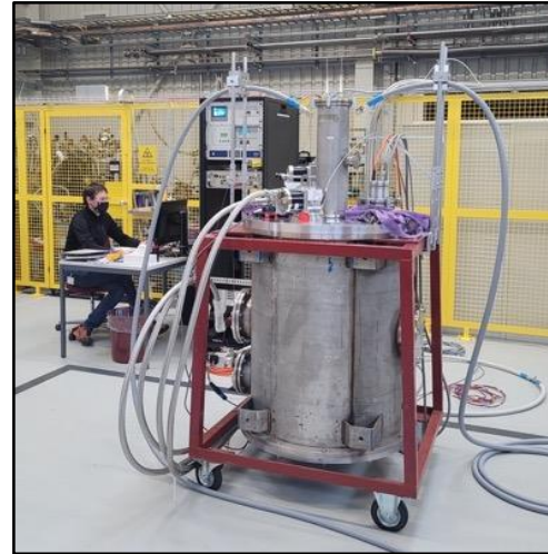
Cryogen-free test station (2 kA)
