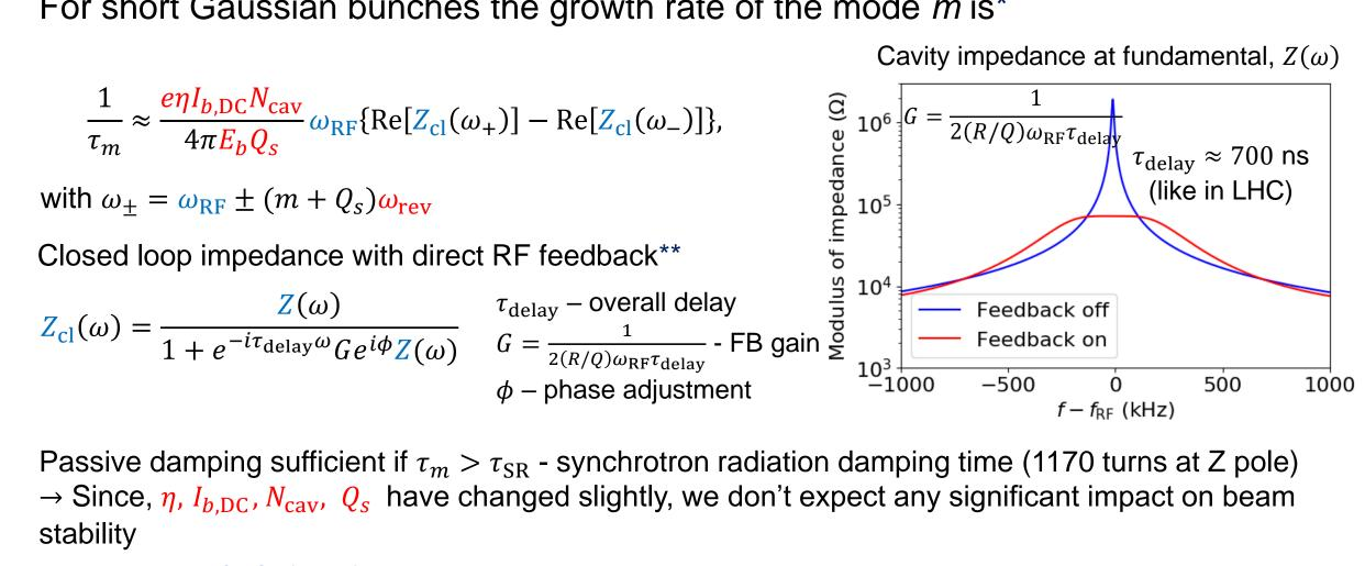
Passive damping sufficient if  $\tau_m > \tau_{SR}$  - synchrotron radiation damping time (1170 turns at Z pole)  $\rightarrow$  Since,  $\eta$ ,  $I_{b,DC}$ ,  $N_{cav}$ ,  $Q_s$  have changed slightly, we don't expect any significant impact on beam stability
