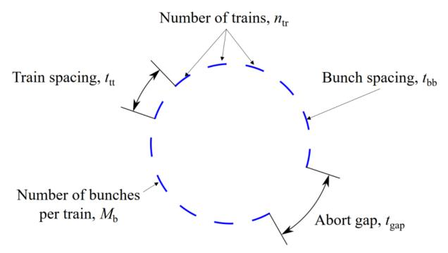
Gaps in machine filling will result in modulation beam parameters (bunch length and phase)
