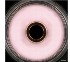
No development of cracks after 5 mounts and thermal shocks
