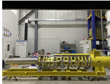
Klystron No. 2 Efficiency 77% (2021)
