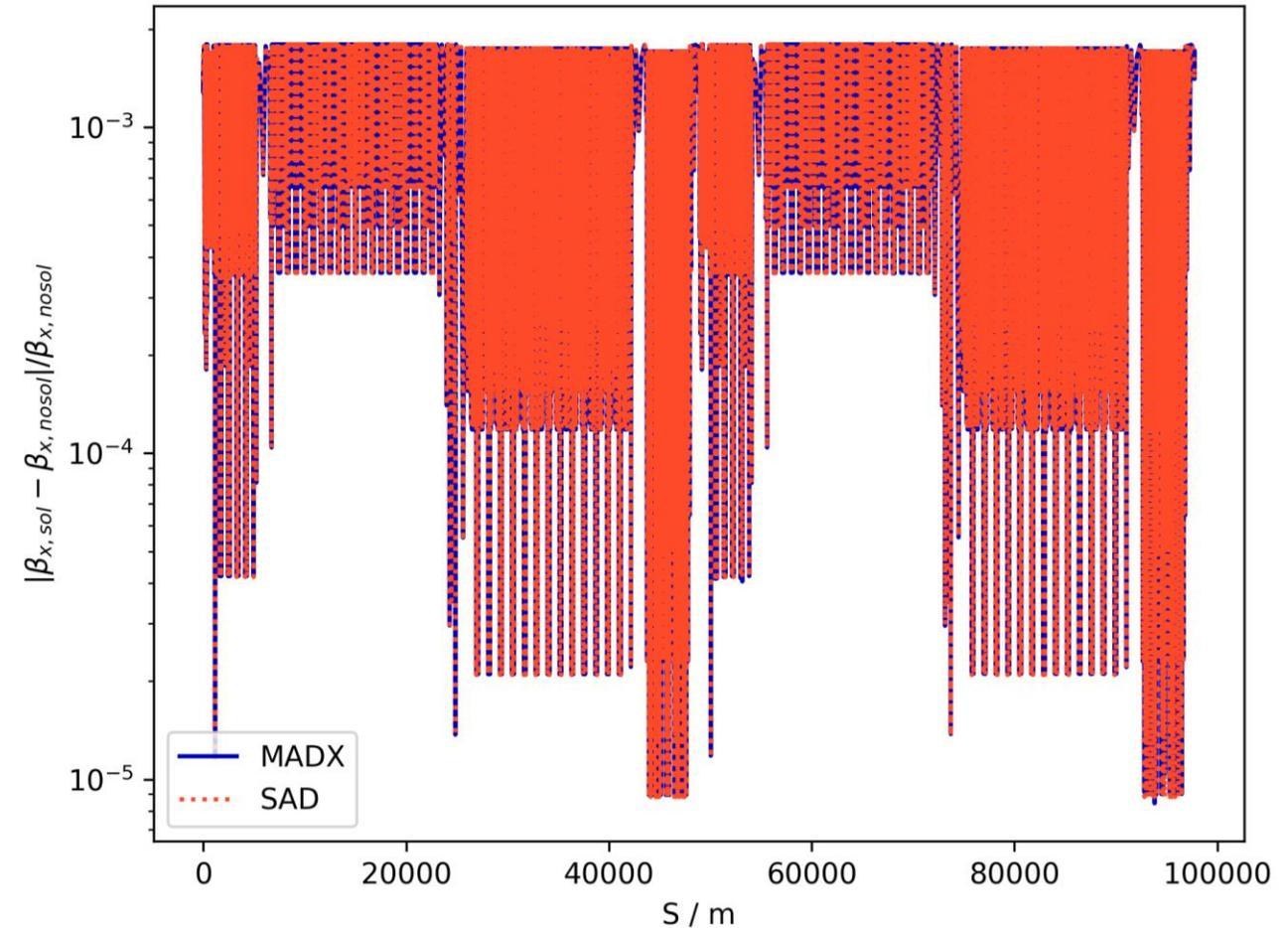
$\beta$ -beating due to turning on tilted solenoid obtained using MAD-X and SAD
