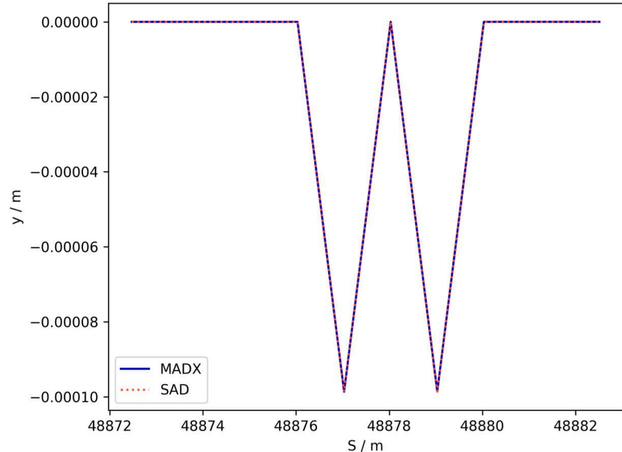
Vertical orbit bump due to tilted solenoid in FCC-ee
