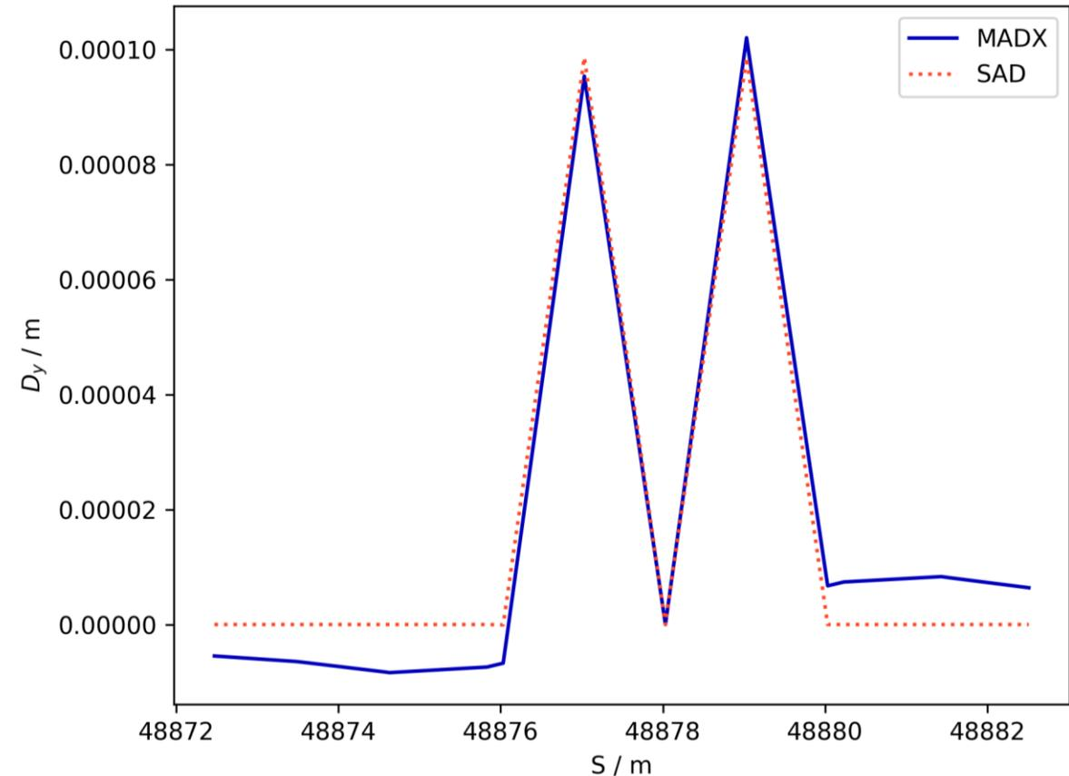
Vertical dispersion due to solenoid/anti-solenoid pair
