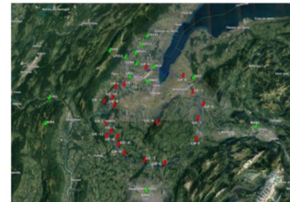
Proposal for newly established (red) and existing (green) surface geodetic points (note: locations are only approximate and may change).
