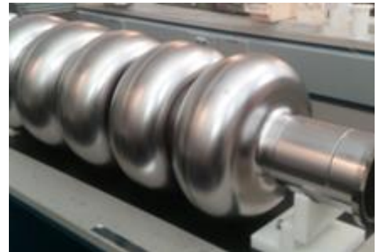
RF Accelerating System
