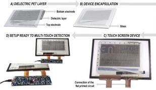
**40 columns** × **28 rows** screen-printed flexible touchscreen Multi-touch capabilities and fast signal processing
