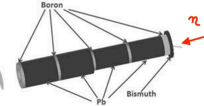
Bi scatter off some fast neutrons, minimise the gamma rays background B high neutron radiative capture cross section
