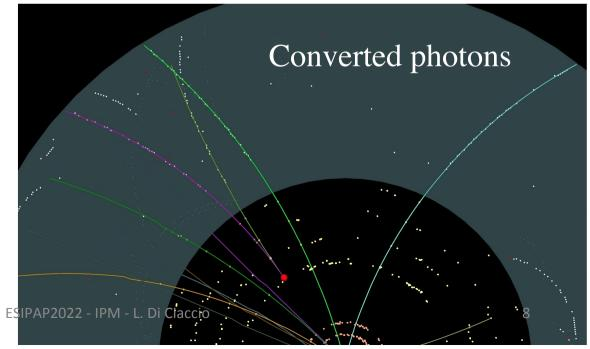
Thanks to photon conversion it is possible to make a radiography of the detector : compare data & MC ← important!
