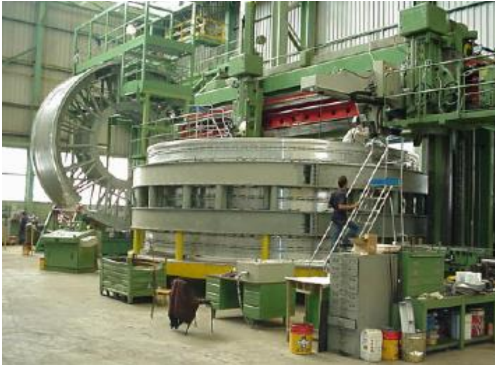
Support cylinder manufacturing, 5 units
