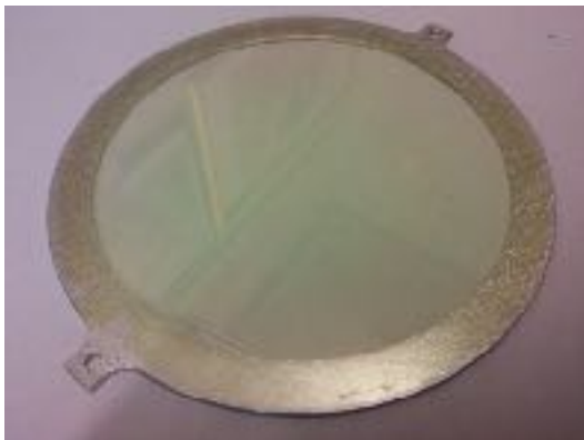
Empty polyimide backing glued to the mounting Al ring
