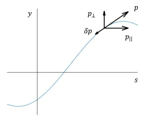
In the RF cavity, the accelerating is purely in the longitudinal direction. As such, only the longitudinal component of the particle's momentum changes, giving rise to a change in the angle of the trajectory. This is the source of the damping in the vertical plane.
