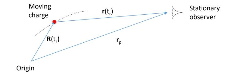
If the charge was at point **R** at the time of emission, then due to the time it takes for the radiation to propagate the distance  $\mathbf{r} = |\mathbf{r}_p - \mathbf{R}|$ , the *actual* time of emission (t<sub>r</sub>) will have been
