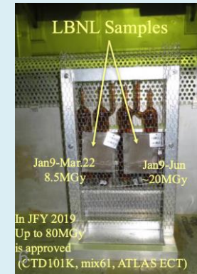
Radiation impacts on magnet materials
