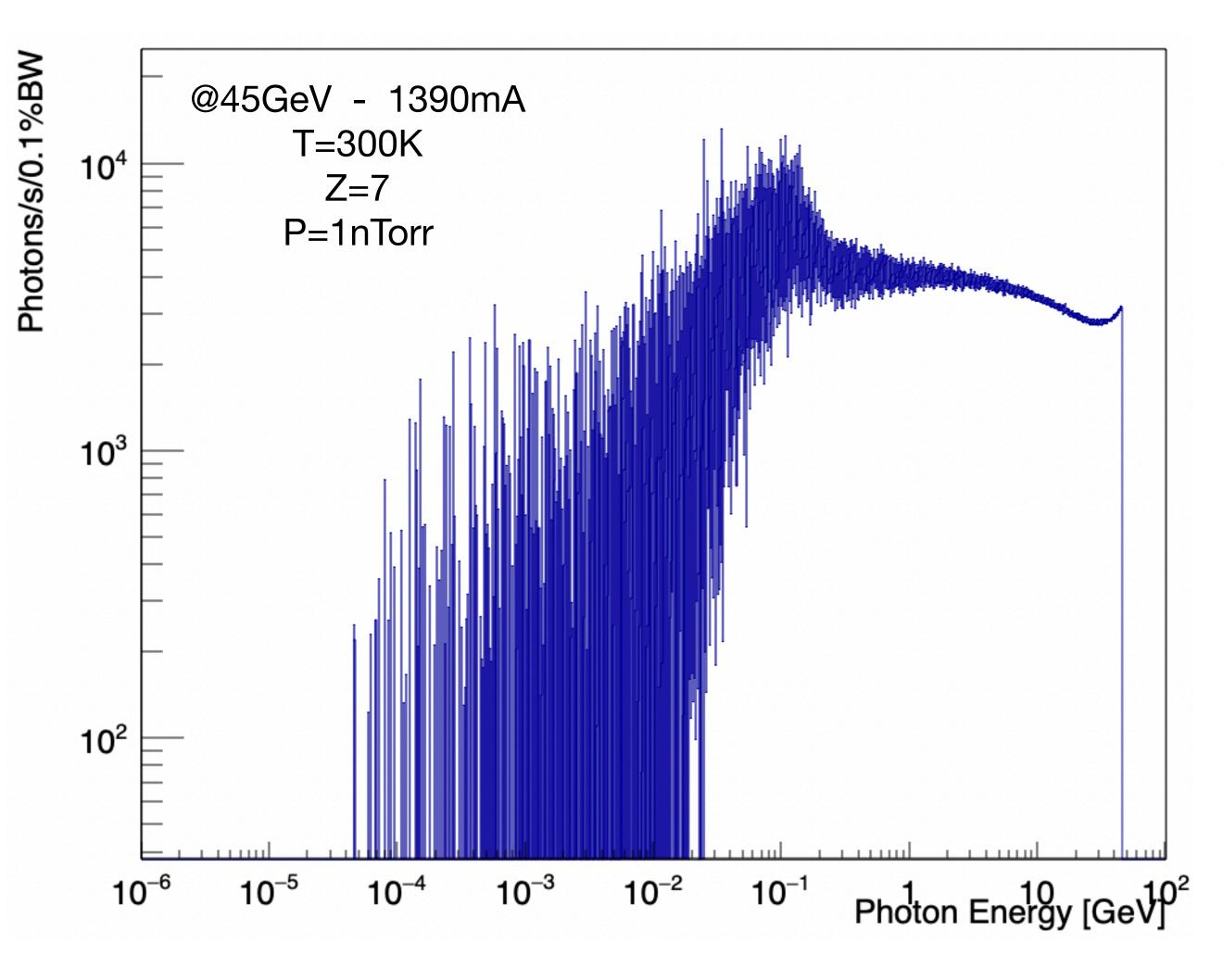
Also the Bremsstrahlung radiation produced by the **inelastic scattering** of the beam particles with **residual gas** in the beam pipe constitutes an unavoidable source of background for this monitor.
