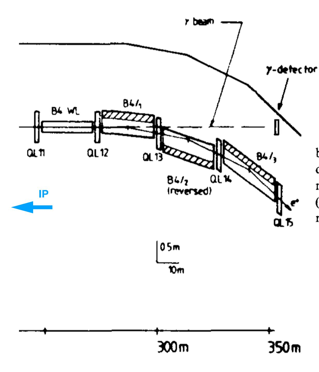
Fast measurement of luminosity at LEP by detecting the single bremsstrahlung photons
