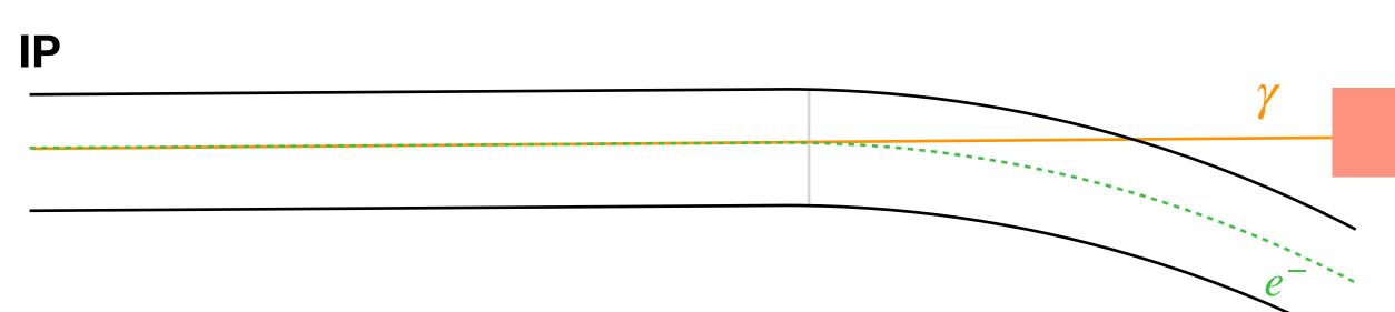
The direction and intensity of the **beam-beam kick** are proportional to the offset between the beams. Because the radiation is produced collinear to the beams, it will carry the information of the offset. This radiation is emitted at **very low angles** and will hit the beam pipe at the **first dipole downstream**.
