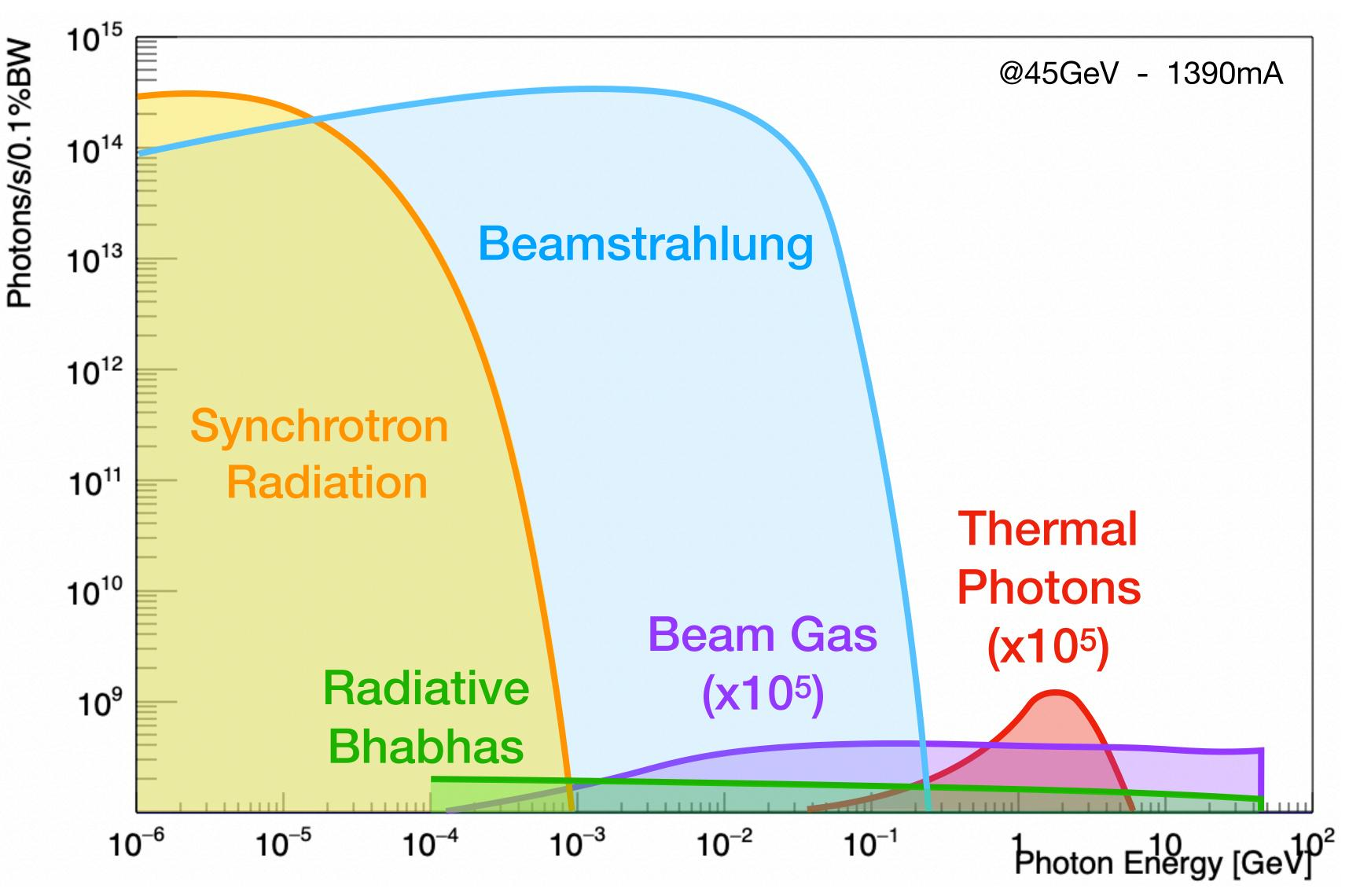
The comparison of the photon flux for the different sources shows that **beamstrahlung** might be a viable signal in the **multi-MeV range**, as its spectrum extends further compared to the synchrotron radiation.
