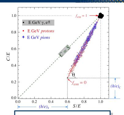
Energy measured from scintillation channel vs Čerenkov channel for EM particle,  $\pi \& p$
